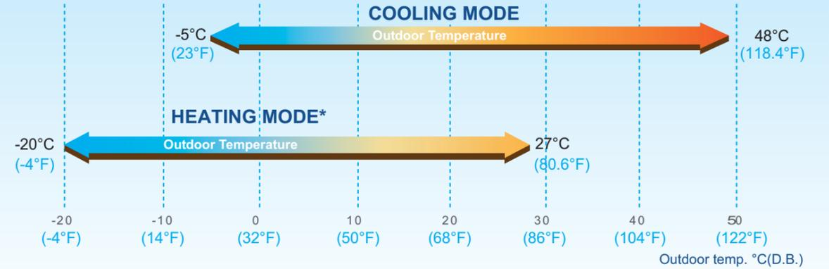
The V4+ series system operates stably at extreme temperatures ranging from -20°C(-4°F) to 48°C(118.4°F). \*V4 Plus C system is without HEATING MODE.
