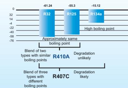
Making continuous efforts to stay eco-friendly, Midea's air conditioners use R-410A, an environmentally friendly refrigerant to help rid the air of pollutants and restrain the use of materials with high global warming potential (GWP). Incorporating the Energy efficient, non-ozone-depleting R410A refrigerant in air conditioning systems delivers multiple benefits:
