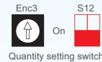
The quantity of indoor units should be exactly set on the outdoor PCB, once some indoor units miscommunicate with outdoor units during system running, the outdoor units will stop and display the fault code "H7". This can prevent compressor from liquid hammer caused by dropped indoor units with EXV unclosed.
