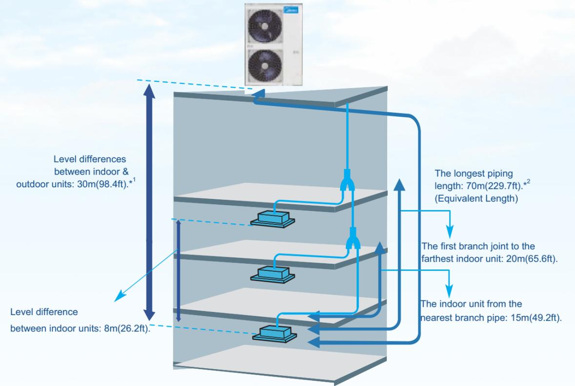
Note:\*1.when outdoor unit up level difference is 30m.,when outdoor unit down level difference is 20m(65.6ft).
